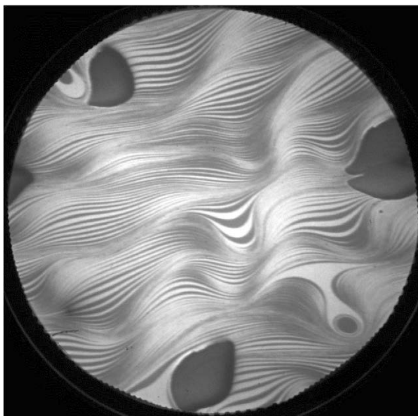
LEEM image selected for the catalogue and exhibition FOTCIENCIA17. Field of view is 20 micrometers and it shows a Ru(0001) surface imaged in dark-field mode. It contains three regions of epitaxial graphene. Atomic terraces are separated by monoatomic steps and present an alternating black-white contrast.
