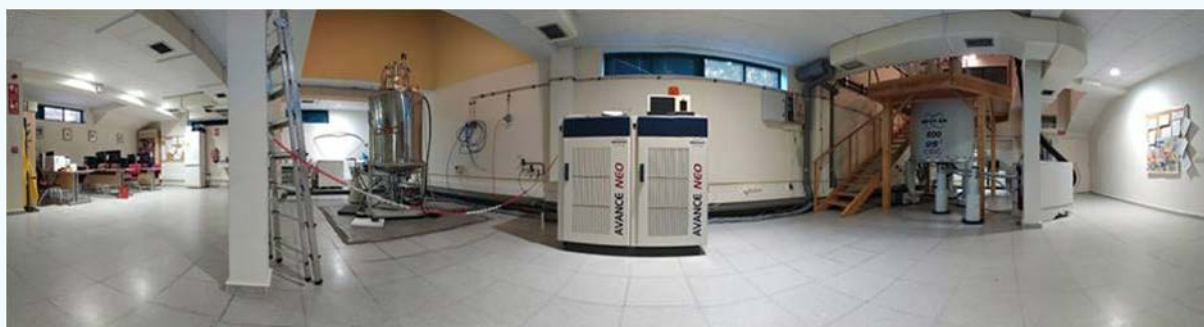
LMR lab. From left to right, the work stations, the Magnet Oxford 14.1T of the 600 MHz NMR spectrometer, the AVANCE NEO consoles of the two NMR spectrometers, and the Magnet Bruker US2 18.8T of the 800 MHz NMR spectrometer.
