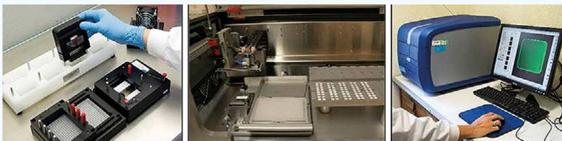
Microarray platform. From left to right, manual contact-system for microarray printing, non-contact microarray robot, and microarray scanner.
