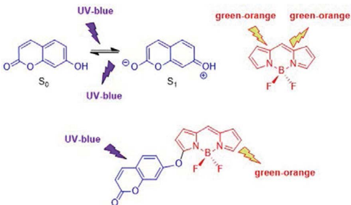
Figure 1: Simple 7-hydroxycoumarin (blue) and BODIPY (red) chromophores, and a hybrid system based on them, indicating the absorption and emission regions of each compound.
