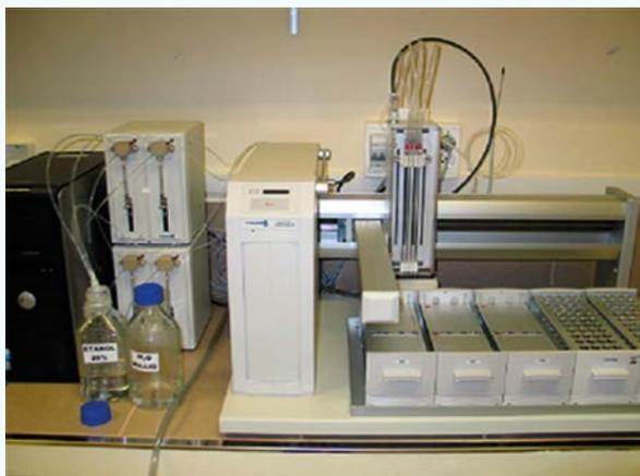
Robot Liquid Handler Quad-Z 215, Gilson Inc.
