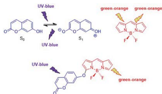
Figure 6. Simple 7-hydroxycoumarin (blue) and BODIPY (red) chromophores, and a hybrid system based on them, indicating the absorption and emission regions of each compound.
