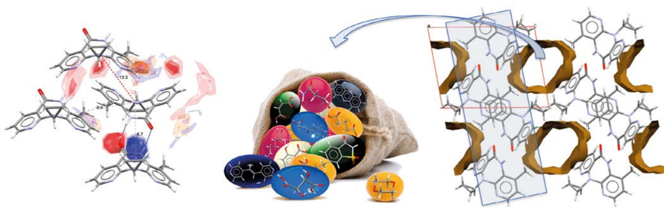
Figure 7. Left: Full Interaction Maps (FIMs) calculated around NVP molecule with three specific probe types: Uncharged NH Nitrogen (blue), Carbonyl Oxygen (red) and Aromatic CH Carbon (yellow). Right: Repetitive packing motif of NVP showing the voids that are occupied for coformers.
